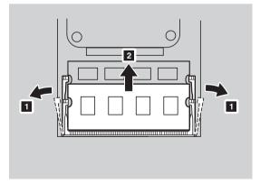
Align the notch of the DDR3 SDRAM with the protrusion of the socket and gently insert the DDR3 SDRAM into the socket at a 30-45° angle. 8 Push the DDR3 SDRAM inward toward the socket until the latches on both edges of the socket are pushed into the closed position.
